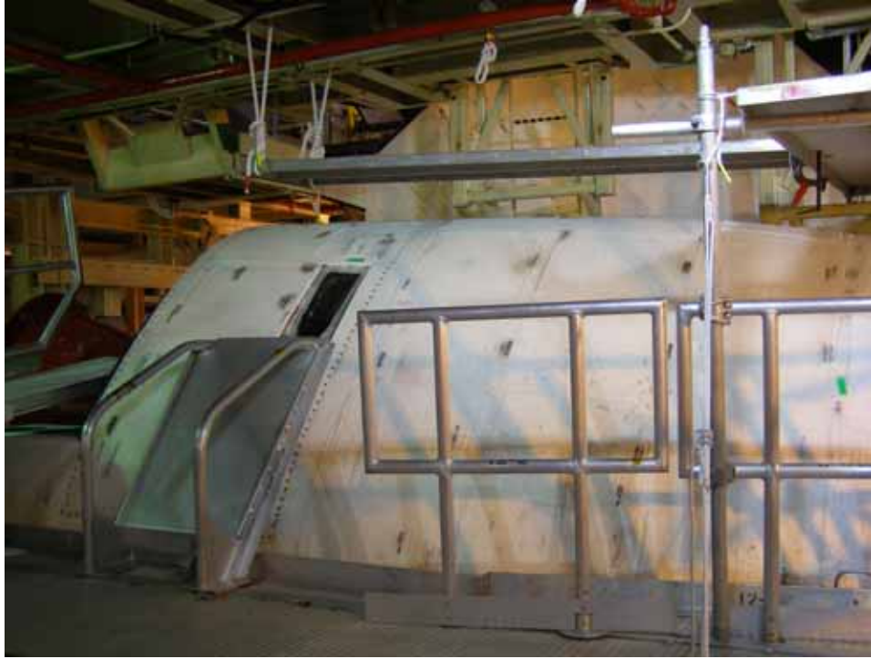
Photo 7. Orbiter Processing Facility High Bay 3, OMS pod with moveable platform. (Source: Archaeological Consultants, Inc., 2006)
