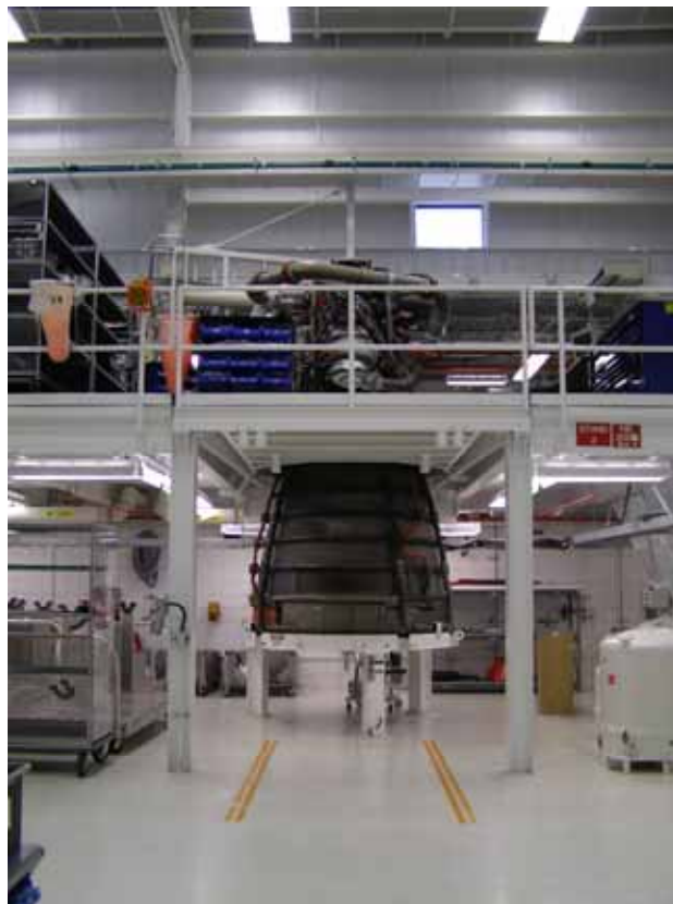
Photo 10. Space Shuttle Main Engine Facility at OPF High Bay 3, vertical stand. (Source: Archaeological Consultants, Inc., 2006)
