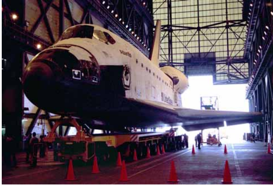
Photo 11. Atlantis being brought into VAB on orbiter transporter, 1997. (Source: NASA John F. Kennedy Space Center, 97PC-1226)
