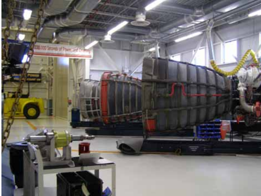
Photo 11. Space Shuttle Main Engine Facility at OPF High Bay 3, horizontal stand area. (Source: Archaeological Consultants, Inc., 2006)
