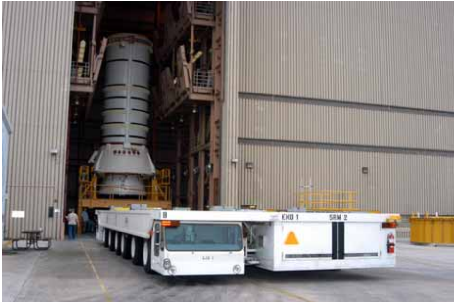
Photo 11. Preparing to move Aft Skirt and SRB lower segment to VAB, 2004. (Source: NASA John F. Kennedy Space Center, KSC-04PD-2358)
