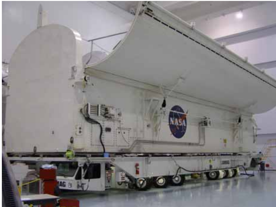
Photo 1. Payload Canister on Canister Transporter in the Space Shuttle Processing Facility. (Source: Archaeological Consultants, Inc., 2006)
