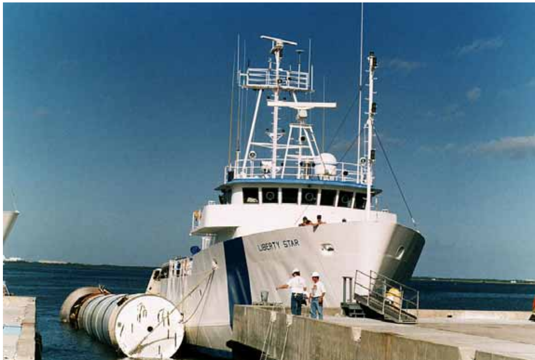
Photo 4. Liberty Star arriving at Hangar AF with spent SRB, post-launch. (Source: NASA John F. Kennedy Space Center, 81PC-0394)
