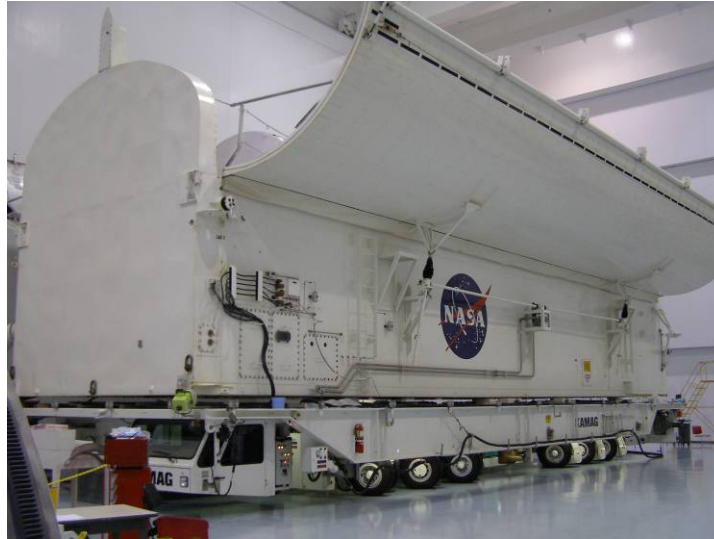
Photo 6.39. Orbiter Payload Canister on Canister Transporter in the Space Shuttle Processing Facility. (Source: Archaeological Consultants, Inc., 2006)
