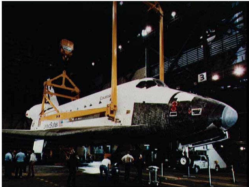
Photo 9. Columbia being fitted into sling for rotation in VAB, 1982. (Source: NASA Lyndon B. Johnson Space Center, S82-27016)
