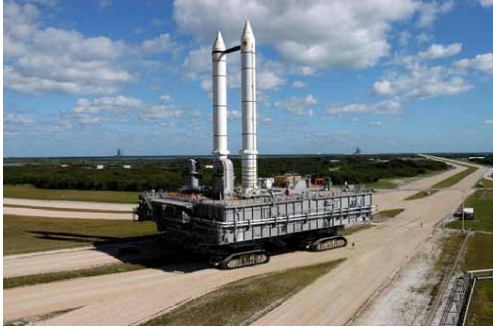
Photo 9. MLP with SRBs at Crawlerway intersection in support of vibration test, 2003. (Source: NASA John F. Kennedy Space Center, KSC-03PD-3159)
