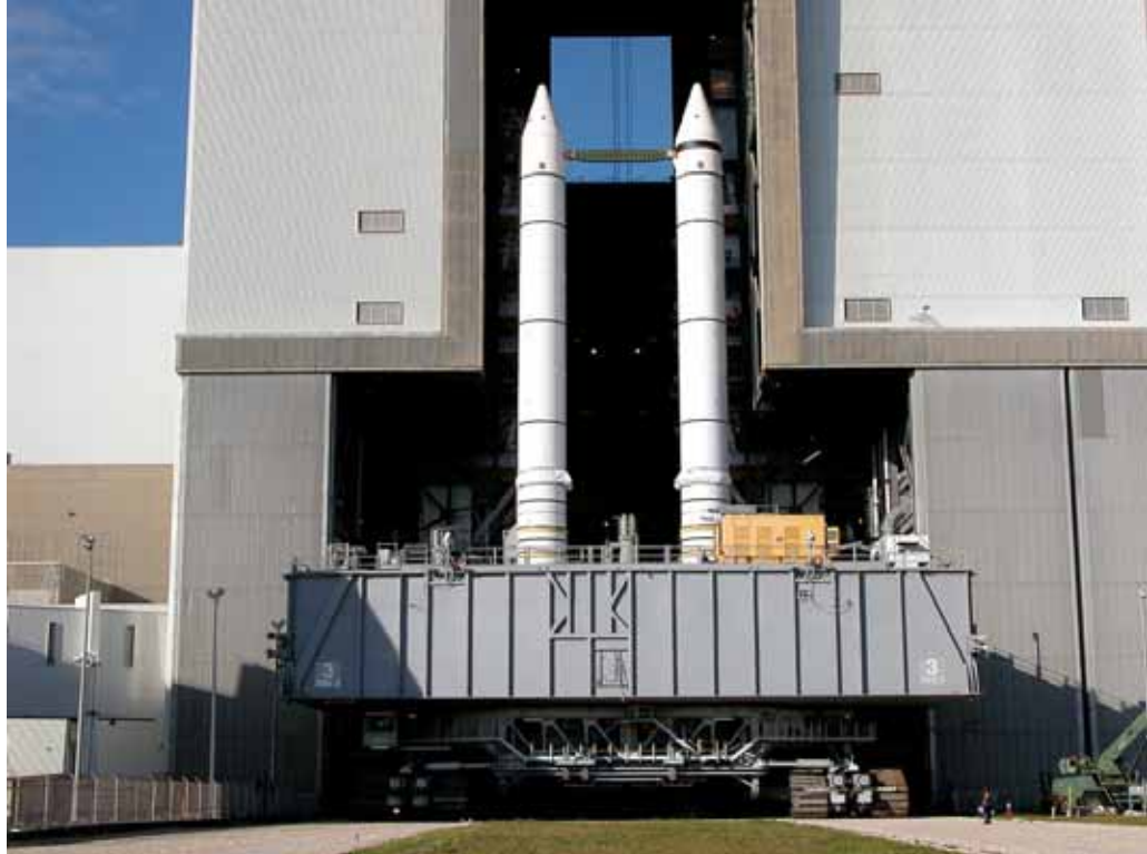
Photo 7. Crawler Transporter carrying MLP with SRBs out of VAB, 2003. (Source: NASA John F. Kennedy Space Center, KSC-03PD-3121)
