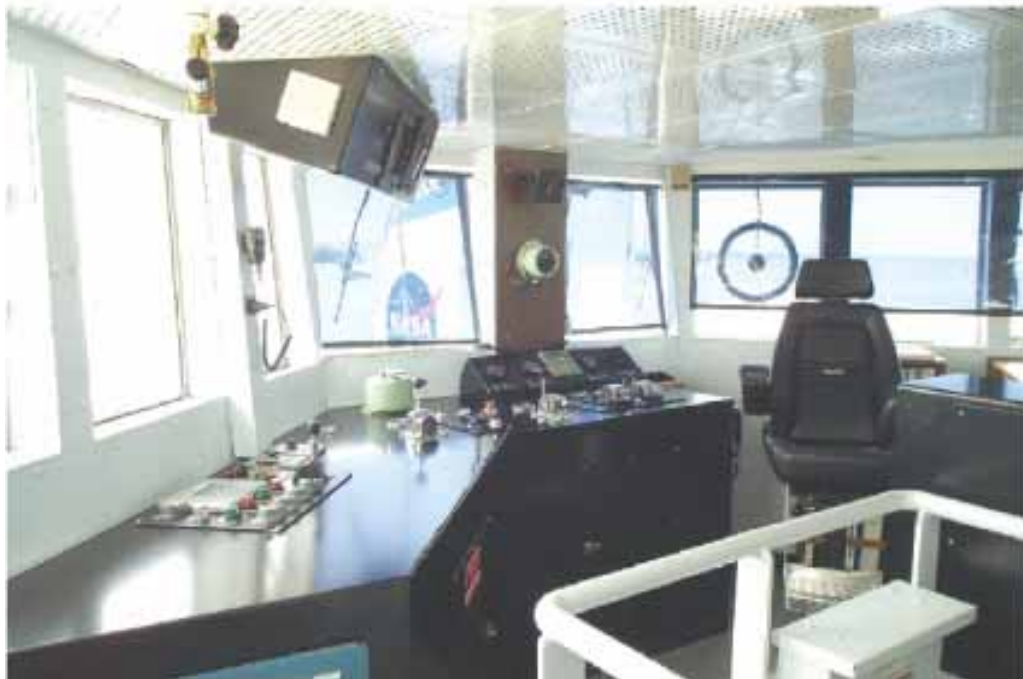
Photo 8. Aft bridge of retrieval vessel, where booster retrieval operations are controlled. (Source: NASAfacts: Space Shuttle Solid Rocket Booster Retrieval Ships )
