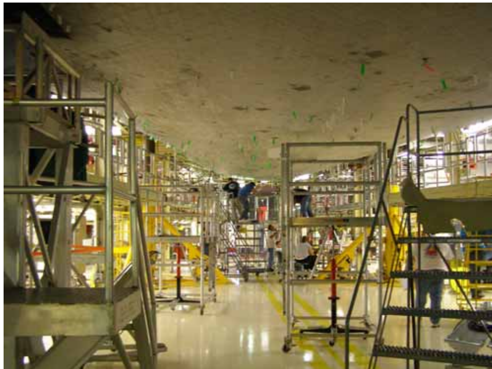
Photo 4. Orbiter Processing Facility High Bay 3, orbiter underside with moveable platforms, looking north. (Source: Archaeological Consultants, Inc., 2006)
