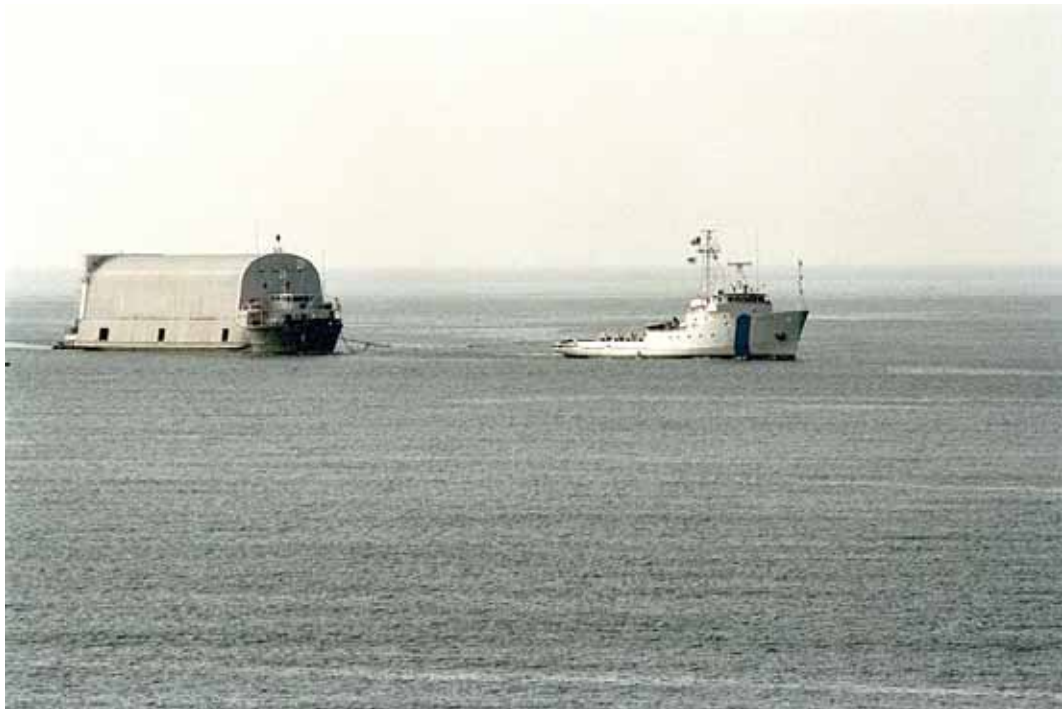
Photo 6. Retrieval Vessel Freedom Star , towing a barge with an external tank. (Source: NASAfacts: Space Shuttle Solid Rocket Booster Retrieval Ships )
