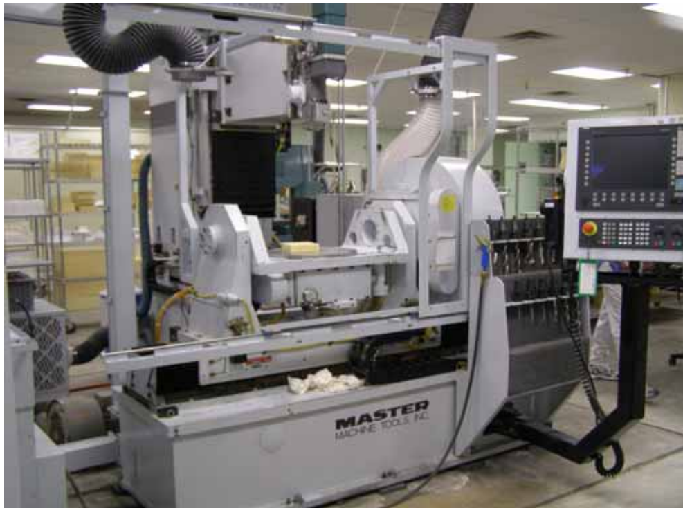
Photo 4. Thermal Protection System Facility, tile cutting machine. (Source: Archaeological Consultants, Inc., 2006)
