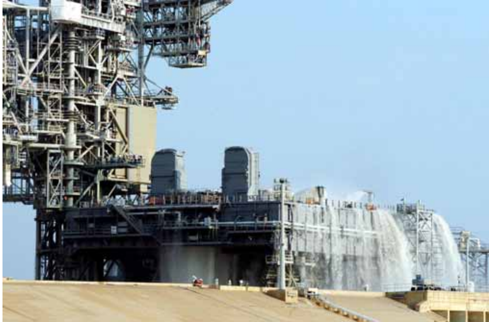
Photo 7. MLP at Launch Pad 39A, during water sound suppression test, 2004. (Source: NASA John F. Kennedy Space Center, KSC-04PD-1068)
